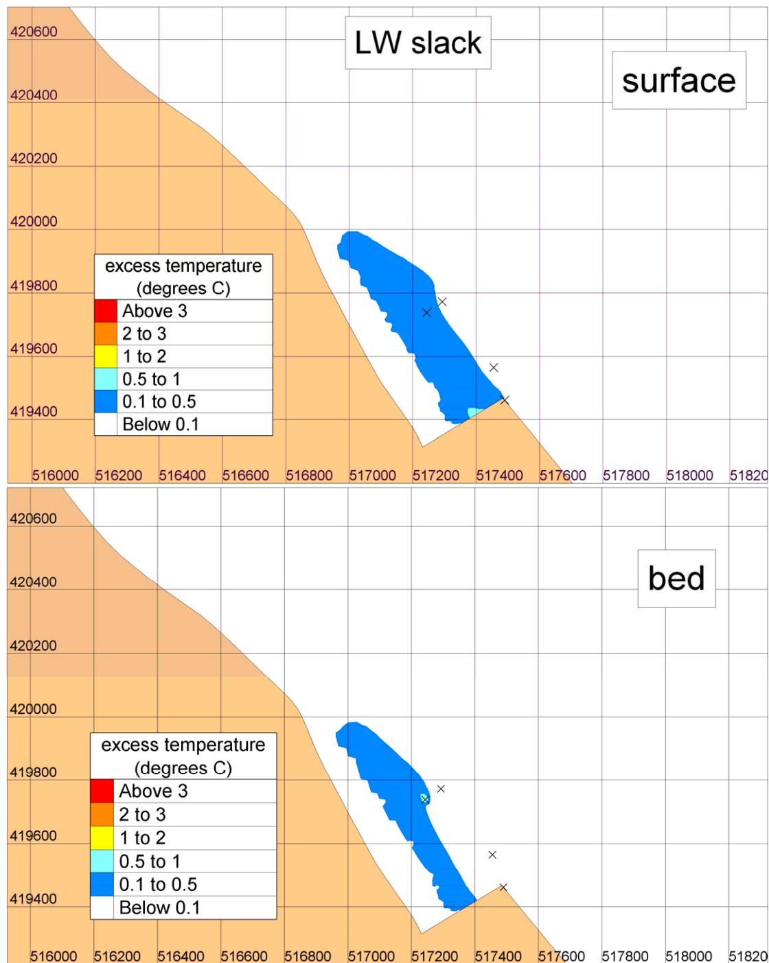
**Figure 2.3 Predicted thermal dispersion patterns at Low Water, final layout with E.ON outfall relocated, spring tide, calm conditions**
